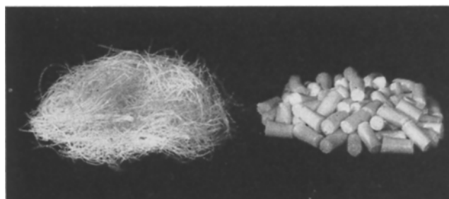
FIG. 6. (Left) Screened soap. (Right) Soap after being pelletized
